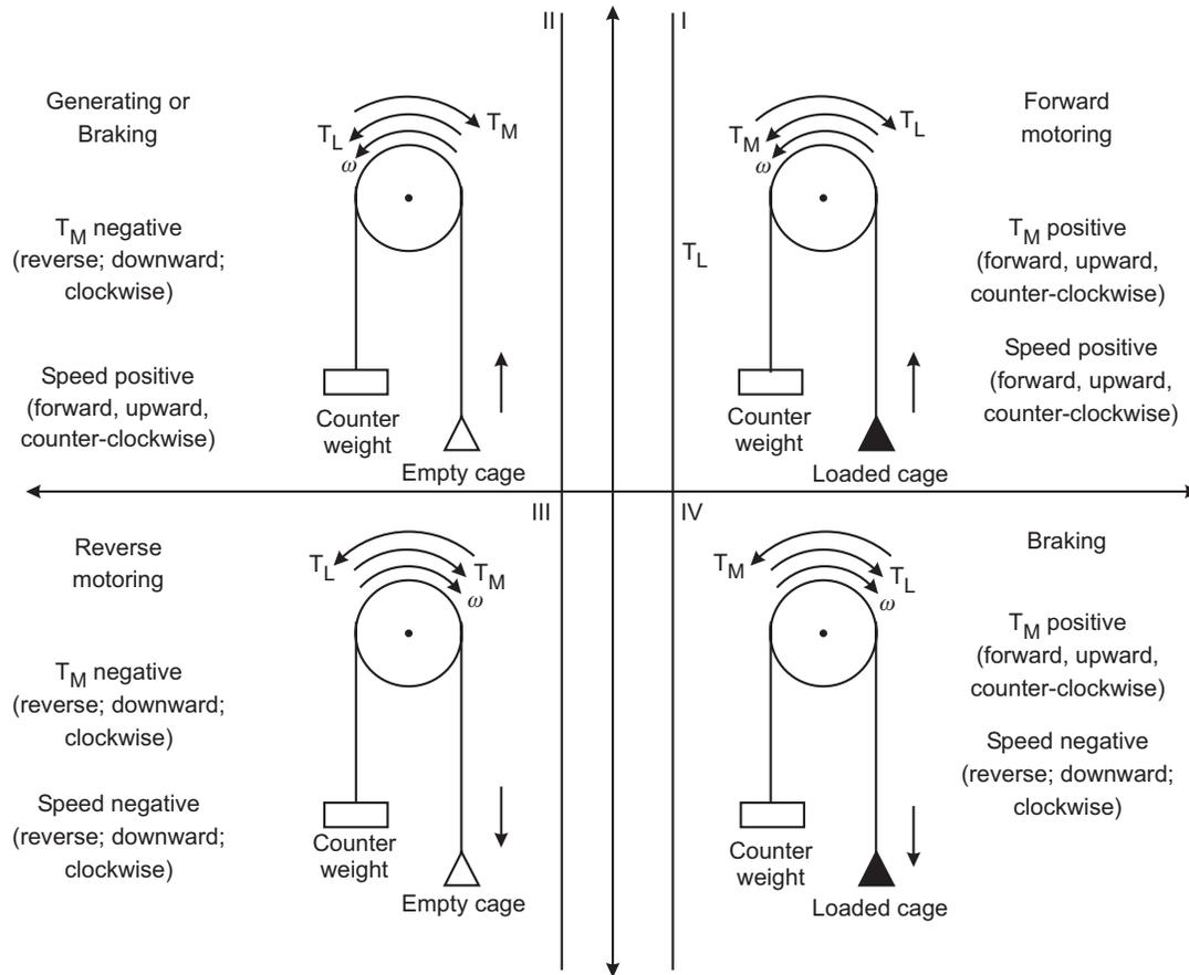
Four quadrant operation of a motor driving a hoist load
