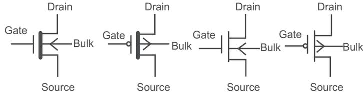
**Figure 1.6:** (a) N and P Depletion MOSFET's. (b) N and P Enhancement MOSFET's
