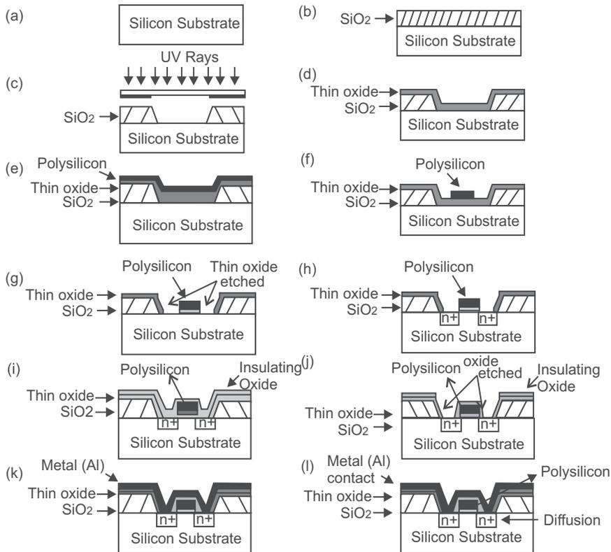
**Figure 1.9:** Fabrication Process of NMOS Device
