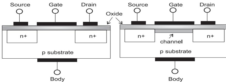
**Figure 1.5:** (a) Enhancement N-type MOSFET (b) Depletion N-type MOSFET
