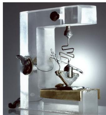
**Figure 1.1:** First Transistor
