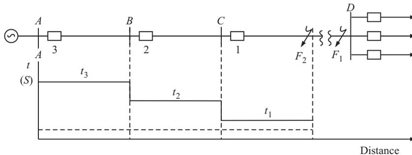
**Figure 7.2:** Time vs distance characteristic of overcurrent protection with acceleration prior to automatic reclosure
