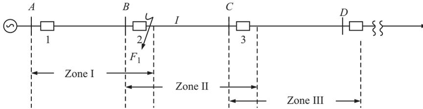
**Figure 7.3:** Overcurrent protection with 'inturn' automatic reclosure
