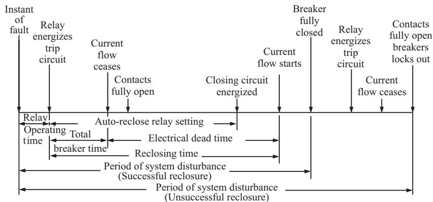
**Figure 7.1:** Auto-reclose cycle for a circuit breaker with a single shot auto-reclose scheme
